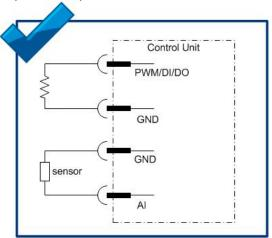
sensors and encoders must be wired according to the closed-loop principle, i.e.
