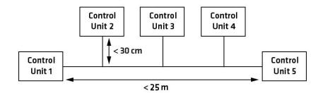
**Example 2**. Control system topology in theory with maximum bus speed (1000 kbit/s); Control Units in traditional bus arrangement. Termination resistor must be connected at control unit 1 and control unit 5. For more information about the bus speeds, refer to CiA DS-102 standard.
