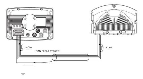
Connection example when there is not a GND pin available in the control unit:
